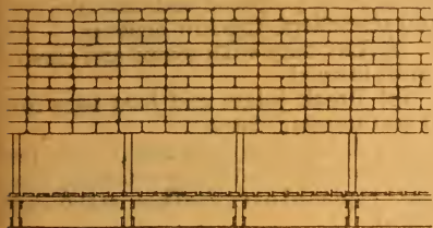
Joints not broken
